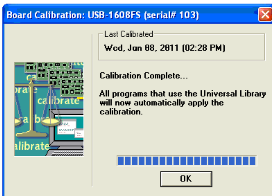
Figure 3. If you get an OK message the USB-interface is correctly installed.
